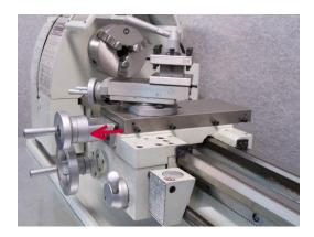
Note the cross slide handwheel dial housing is now flush against the cross slide:
