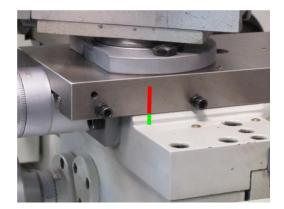
Reposition the cross slide to the rear-most position:
